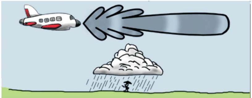
Figure 6-14 Flat-Plate Radar Antenna Beam Patterns
