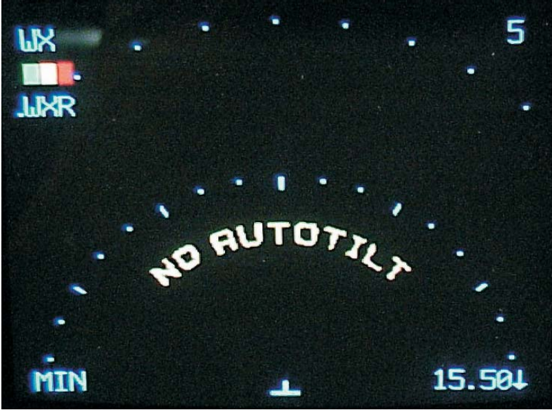
Figure 4-9 Retrofit Automatic Function Fail Annunciation
