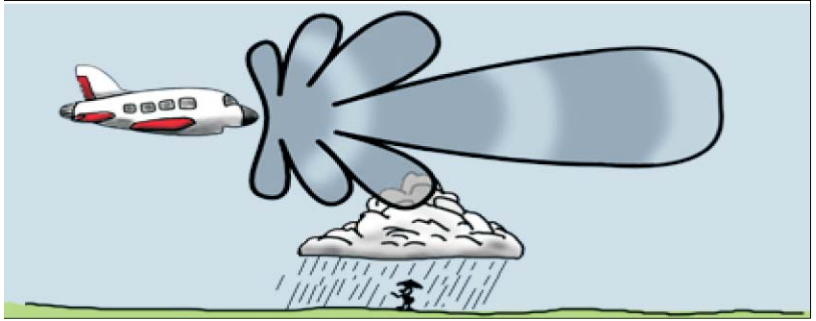
Figure 6-13 Parabolic Radar Antenna Beam Patterns
